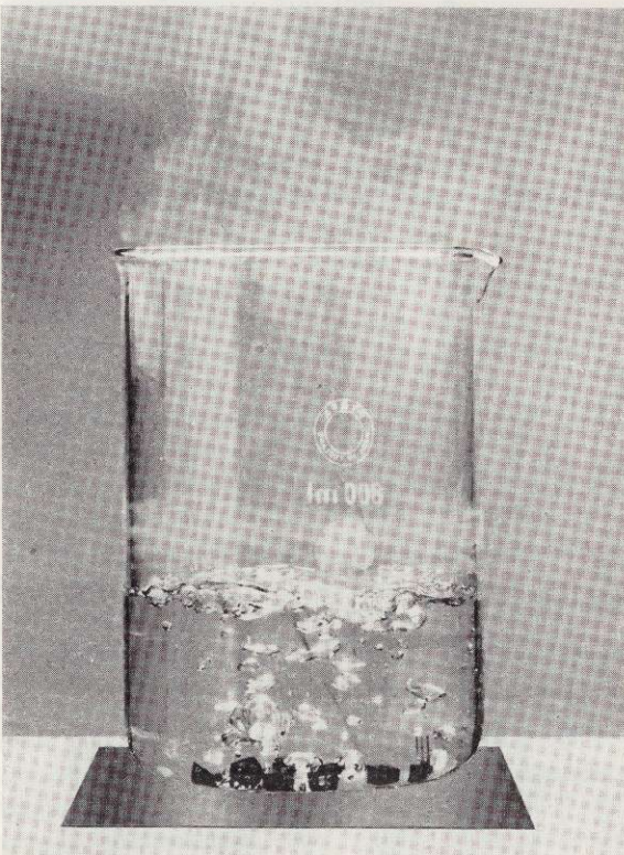
Fig. 16. Lock-fit Transistors immersed in boiling water. Subsequent to the boiling cycle, the Transistors are tested to guarantee positive sealing.
