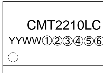
Figure 12. CMT2210LC Top Marking
