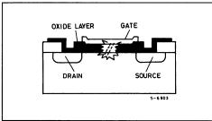
This happens mostly because a charged conductor. typically a person, is radiply discharged through the device.
