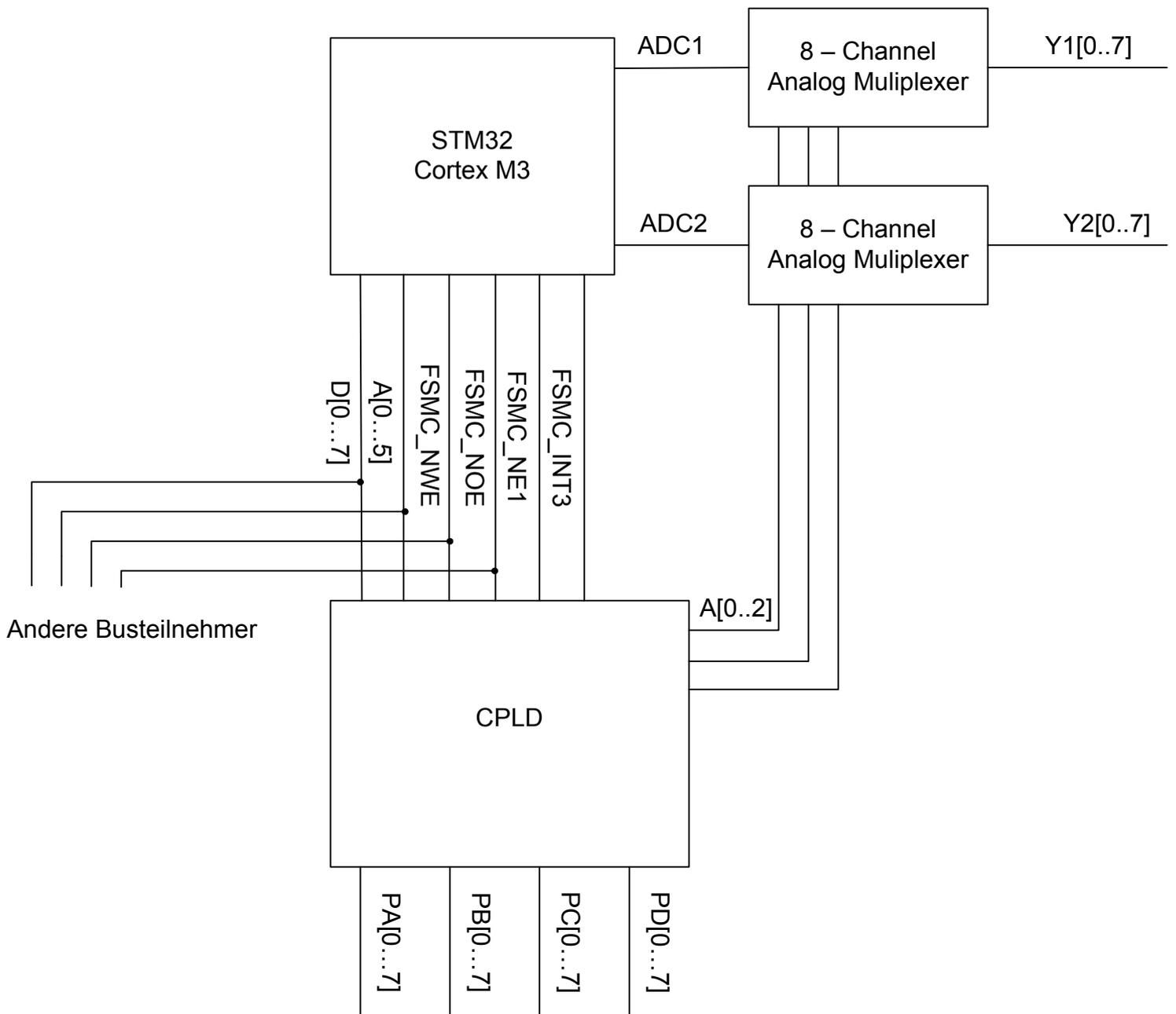
FSMC – Flexible static memory controller
