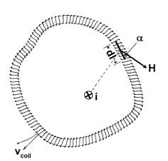
Where dl is a small element of length along the loop, H is the magnetic field and  $\alpha$  is the angle between the direction of the field and the direction of the element.
