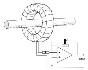
waveform. This combination of coil and integrator provides a system where the output is independent of frequency, which has an accurate phase response, and which can measure complex current waveforms. The output from the integrator can be used with any form of electronic indicating device such as a voltmeter, oscilloscope, protection system or metering equipment.
