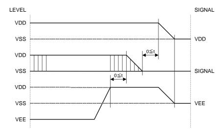
Please maintain the above sequence when turning on and off the power supply of the module. If  $V_{EE}$  is supplied to the module while internal alternate signal for LCD driving (M) is unstable, DC component will be supplied to the LCD panel. This may cause damage the LCD module.
