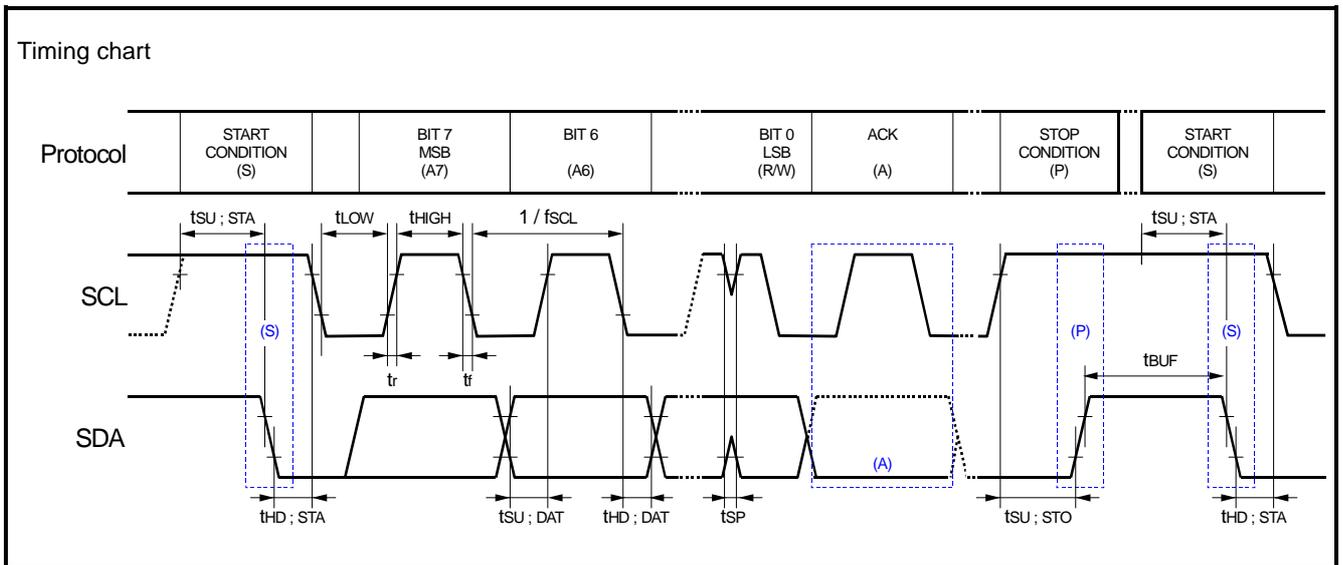
Note : I<sup>2</sup>C access time between a START and a START condition or between a START and a STOP condition to this device must be less than one second.
