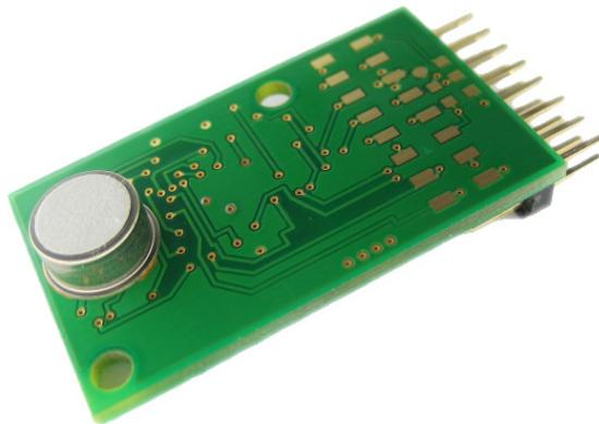
During the first 6 hours of continuous operation (burn-in) the module will display 450ppm, 2.5VDC, 50%PWM. The successful burn-in is saved to the EEPROM, the run-in time after restart is 15min.
