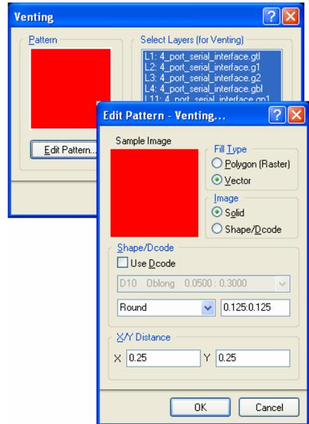
If you created venting when you originally panelized the data, then added ODB++ steps such as coupons, tooling holes, or even flipped or alternate boards, you should refresh the venting pattern. This is achieved by removing venting and then adding it again. Commands for such will appear when you right-click on the step entry for the panel (`campanel`), in the **Steps** tab of the **CAMtastic** panel – remember to make the panel step the current step in order for
