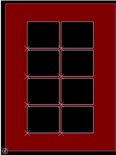
If you created venting when you originally panelized the data, then added ODB++ steps such as coupons, tooling holes, or even flipped or alternate boards, you should refresh the venting pattern. This is achieved by removing venting and then adding it again. Commands for such will appear when you right-click on the step entry for the panel (`campanel`), in the **Steps** tab of the **CAMtastic** panel – remember to make the panel step the current step in order for these commands to become active.
