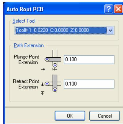
You may proceed to add tabs along the routing path, which retracts the drill from the panel and moves ahead along the path a specified distance before plunging in again. Placing routing tabs is analogous to jump-scoring segments: they leave boards fully connected to the panel at certain points, ready to be broken away at a later time.
