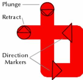
Several considerations are important when preparing routing information. These include the size and shape of the drill tool, and the rout path, along with its plunge and retract points.
