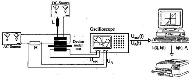
Fig. 4: Measurement setup
