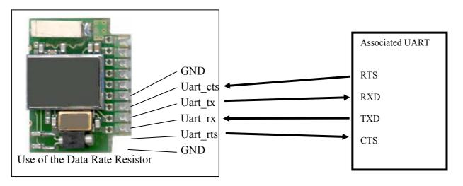
Data Rate Resistor (red component) The purpose of this resistor is to access the ARF32 module by forcing the UART data rate in case of bad "Non Volatile Settings" programming during test and evaluation.
