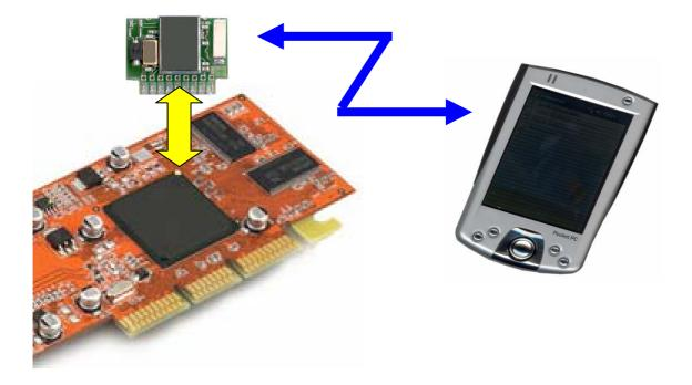
The ARF32 module fully complies with the V1.1 Bluetooth<sup>®</sup> standard and data rate goes up to 723 kbps. Data exchange and set-up are only done through an UART data port, under SPP profile. A miniature antenna is integrated.
