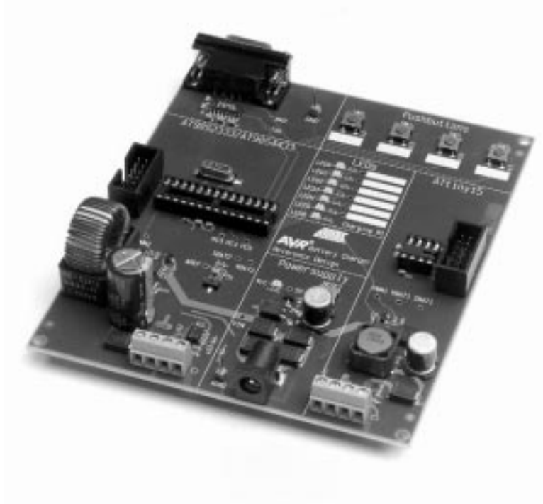
Figure 1. Battery charger reference design board
