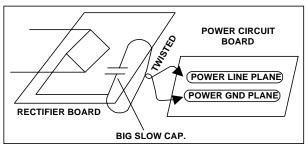
Figure 7. Power Bypass Capacitor
