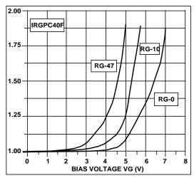
Figure 19. Turn-on losses vs. VG
