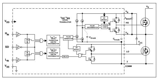
Figure 2. Block Diagram of the IR2110
