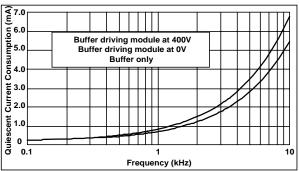
Figure 14. Current consumption vs. frequency
