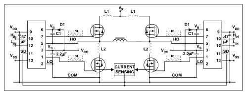
Figure 29. Typical implementation of all H-Bridge with cycle-by-cycle current mode control
