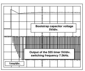
Figure 17. Waveform at start-up.
