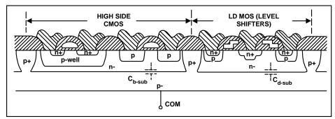
Figure 3. Silicon crossection showing the parasitic capacitances.
