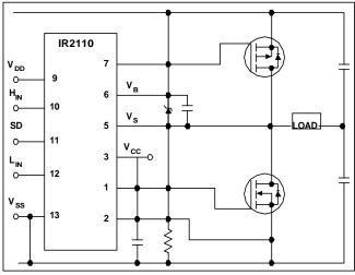
Figure 33. IR2110 driving a high side P-Channel
