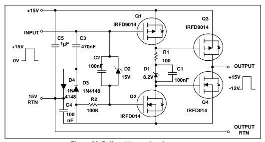
Figure 20. Buffer with negative charge pump
