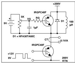
Figure 18. Test circuit
