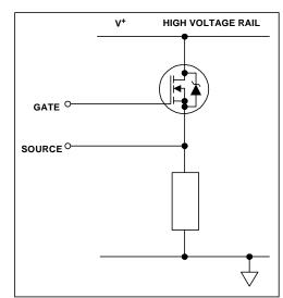
**Figure 1.** Power MOSFET in high side configuration
