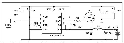
Figure 26. In battery charger applications, the +12V from the output appears at the ½ pin and reduces the voltage across CB at start-up and the undervoltage protection in the IR21XX inhibits the operation.
