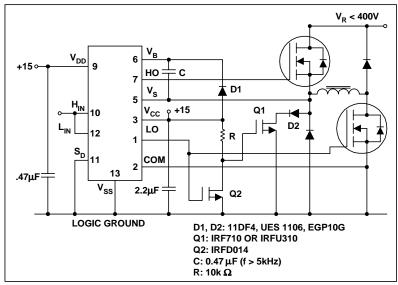
Figure 28. Dual forward converter and switched reluctance motors
