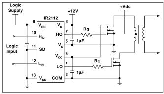
Figure 32. Push Pull Drive Circuit
