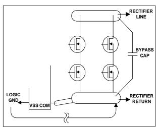
Figure 6. Ground connections and layout
