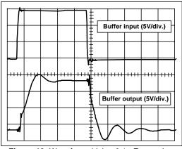
Figure 13. Waveform driving 0.1mF capacitor (250nS/div.)
