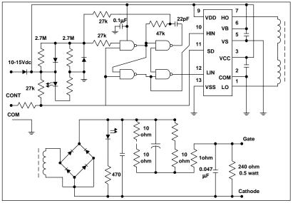
Figure 34. Isolated SCR Gate Drive Circuit
