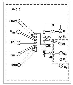
**Figure 10.** IR2110 test circuit Note: Dotted lines represent pads on bottom side of board. V+, GND, D1, S1, D2, S2, terminals have plated through holes
