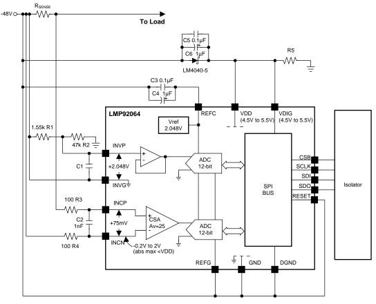
Figure 26. Typical Applications Circuit
