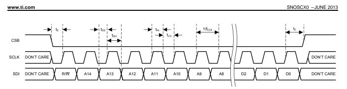
Figure 5. Serial Control Port Write – MSB First, 16-bit Instruction, Timing Measurements
