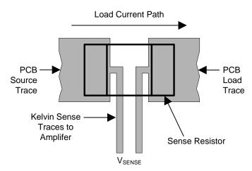
Figure 22. 4-Wire "Kelvin" Sensing Technique
