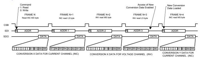
Figure 23. Timing Diagram with Byte Read Frames
