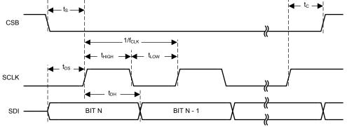
Figure 3. Serial Control Port Timing – Write
