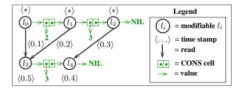
Figure 4: The ADG for an application of filter' to the function fn x => x>2 and the input modifiable list 2::3::nil. The output is the modifiable list 3::nil.
