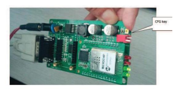
If you don't have the WIFI evaluation board, you can make the CFG pin connect the GND pin 3 Seconds (CFG pin active low)
