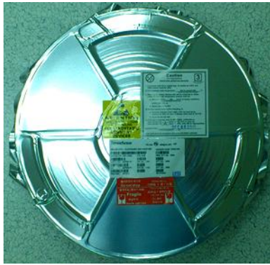
Vacuum-Sealed Moisture Barrier Bag with ESD, MSL3, Caution, and Barcode Labels
