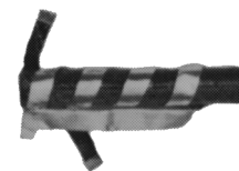
Line Transformer on Ferrite (Figure 30)
