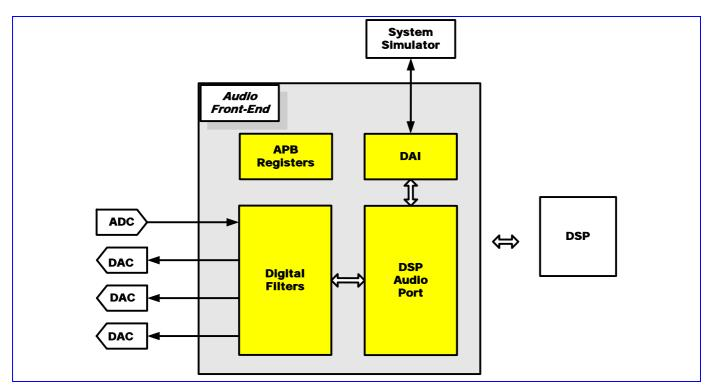
Figure 57 Block diagram of digital circuits of the audio front-end
