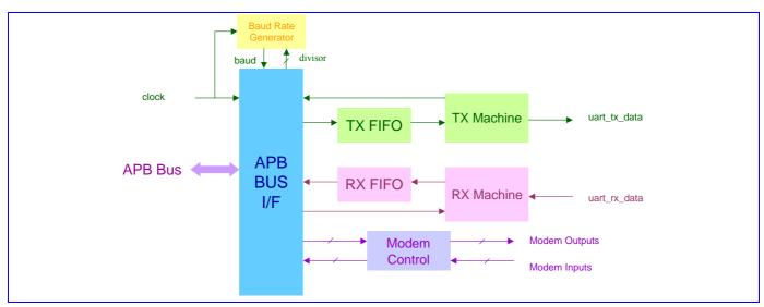
Figure 29 Block Diagram of UART
