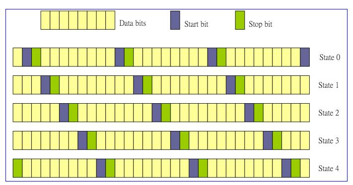
Figure 36 data format conversion of RA0
