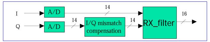
Figure 54 I/Q Mismatch Compensation Block Diagram
