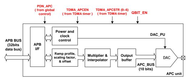
Figure 46 Block diagram of APC unit.
