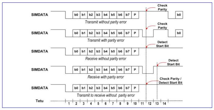
Figure 24 SIM Interface Timing Diagram
