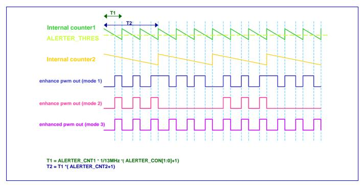
Figure 21 Alerter Waveform
