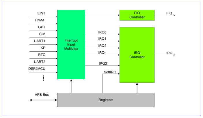
Figure 14 Block Diagram of the Interrupt Controller
