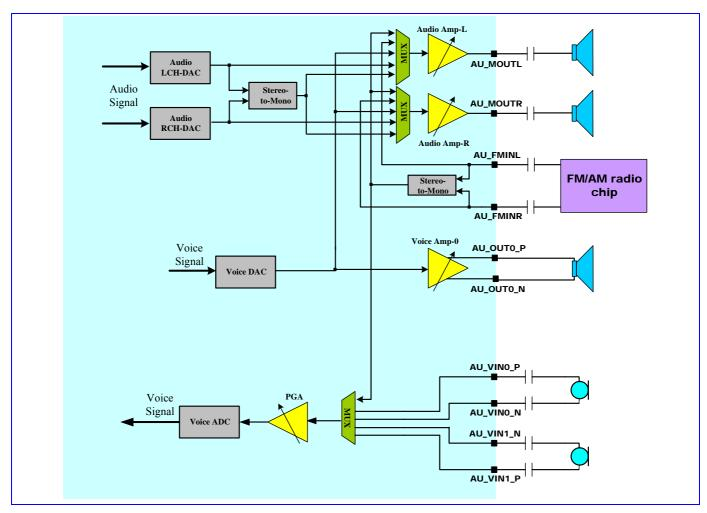
Figure 75 Block diagram of audio mixed-signal blocks.
