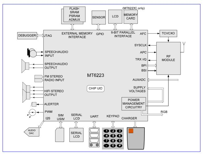
Figure 1 Typical application of MT6223.
