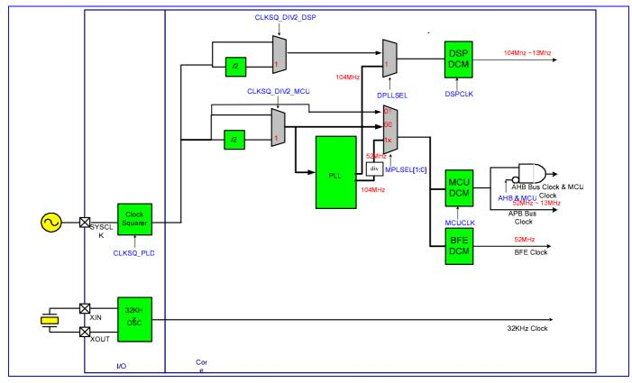
Figure 70 Clock distributions inside the MT6223.
