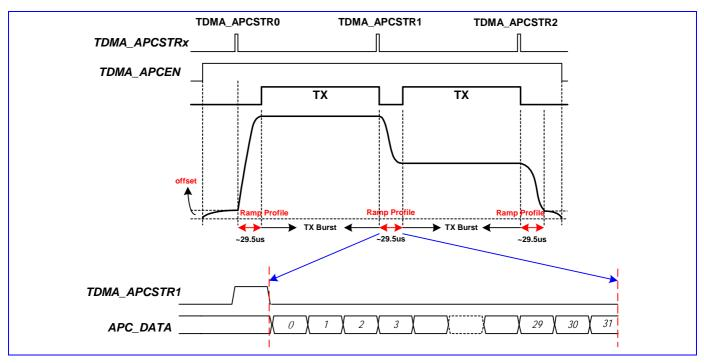
Figure 49 Timing diagram of the APC ramping.
