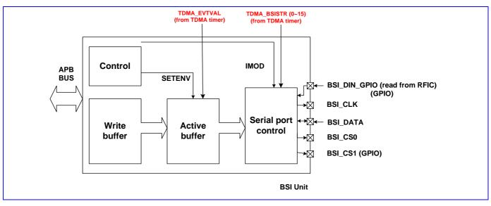
Figure 43 Block diagram of BSI unit.
