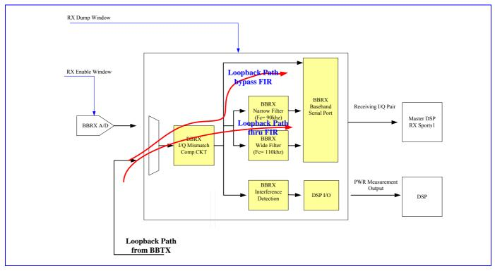
Figure 53 Block diagram of RX path
