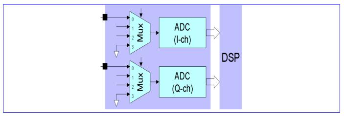
Figure 79 Downlink ADC Offset Error Measurement
