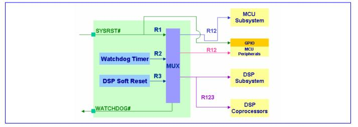
Figure 73 Reset Scheme Used in MT6223
