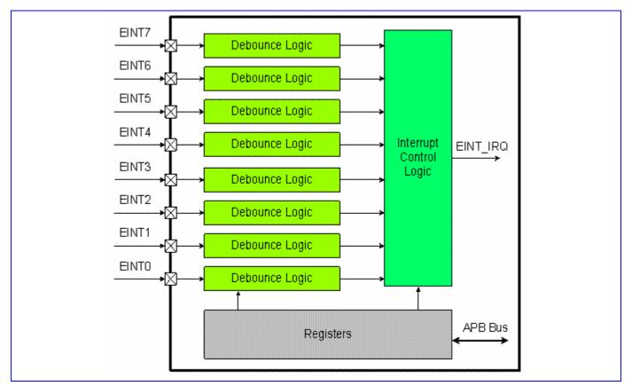
Figure 15 Block diagram of External Interrupt Controller
