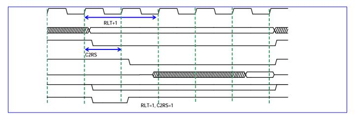
Figure 17 Read Wait State Timing Diagram (ADVR=0)
