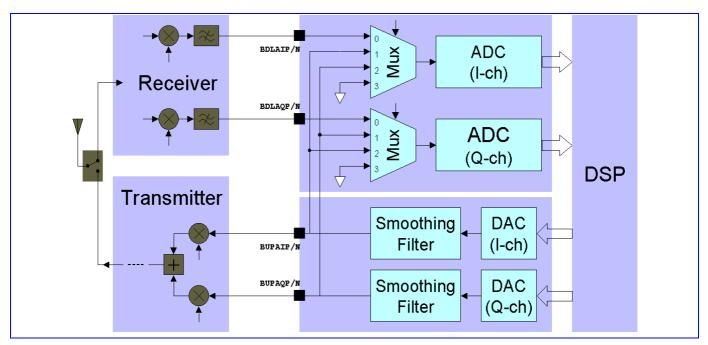
Figure 78 Base-band A/D and D/A Offset and Gain Calibration
