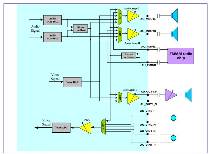
Figure 56 Block diagram of audio front-end
