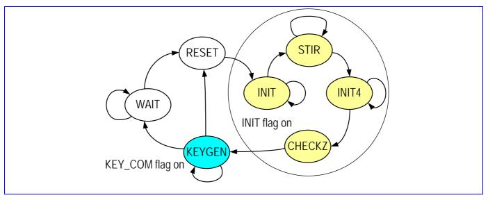
Figure 32 The state diagram of the GCU
