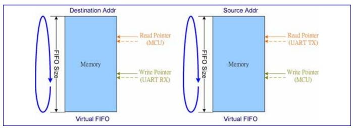
Note that Virtual FIFO DMAs cannot be used as generic DMAs, i.e. DMA1 and DMA4~8.
