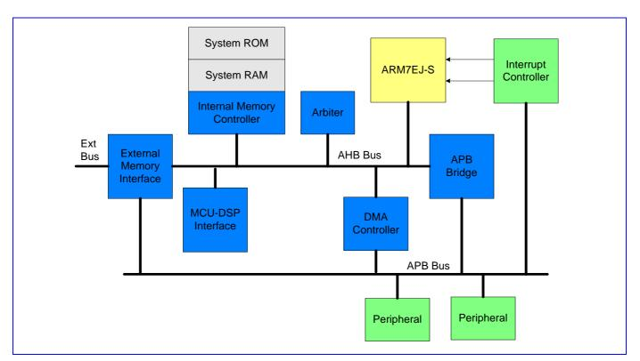
Figure 5 Block Diagram of the Micro-Controller Unit Subsystem in MT6223
