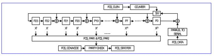
Figure 42 FCS codec circuit.
