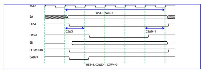
Figure 19 Write Wait State Timing Diagram (ADVW=0)
