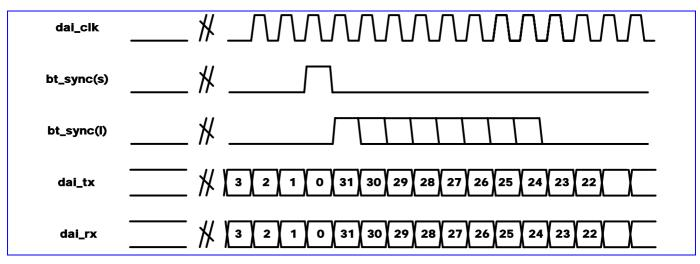
Figure 58 Timing diagram of Bluetooth application
