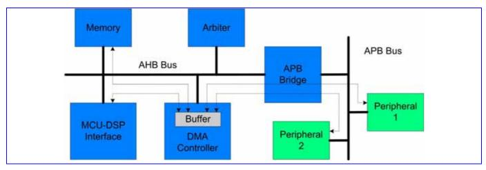
Figure 8 Variety Data Paths of DMA Transfers
