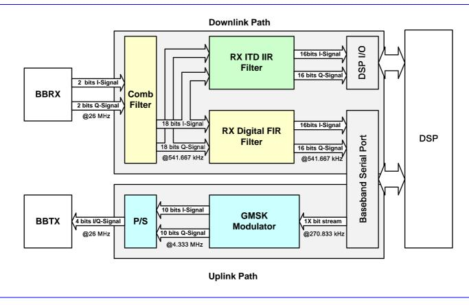
Figure 52 Block Diagram of Baseband Front End
