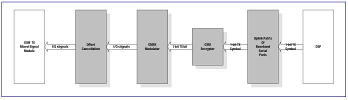
Figure 55 Block Diagram of Uplink Path
