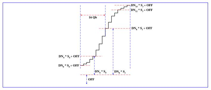
Figure 48 **The timing diagram of the APC ramp.**
