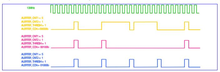
Figure 22 Alerter Output Signal from Enhanced PWM with Register Value Present
