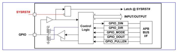
Figure 30 GPIO Block Diagram
