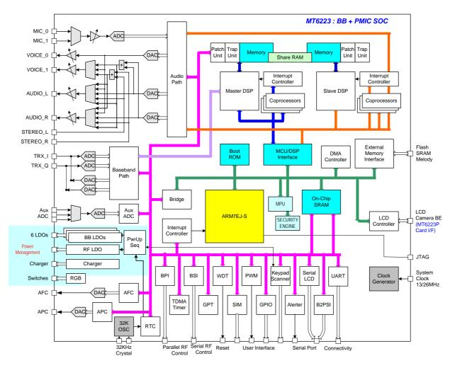
Figure 2 MT6223 block diagram.
