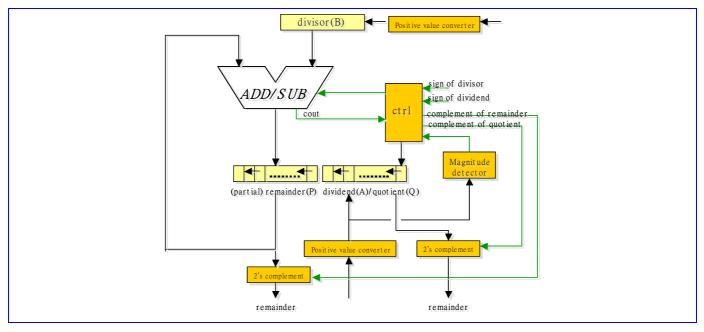
Figure 35 Architecture of radic-2 non-restoring divider for MCU system
