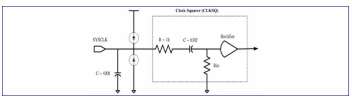
Figure 76 Equivalent circuit of Clock Squarer.
