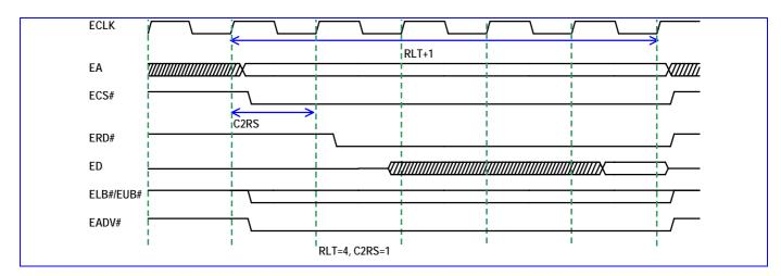
Figure 16 Read Wait State Timing Diagram (ADVR=1)
