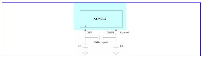
Figure 77 Block diagram of XOSC32
