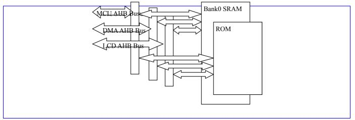
Figure 20: Block Diagram of the Internal Memory Controller
