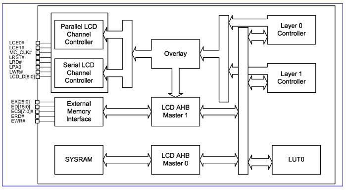
Figure 26 LCD Interface Block Diagram
