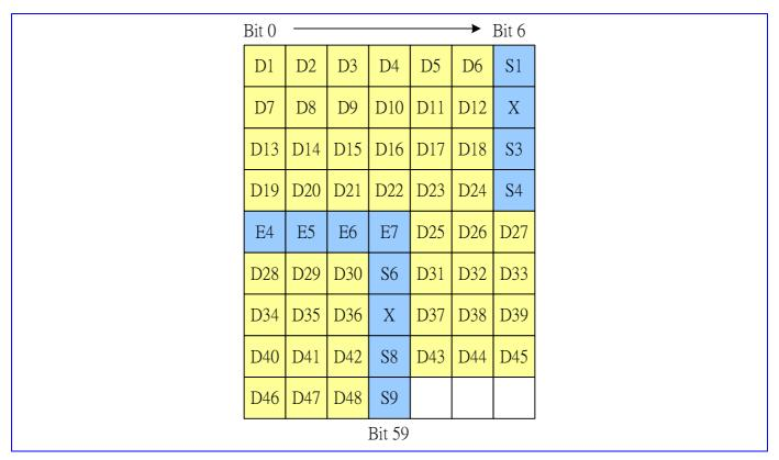
Figure 37 data format conversion for 6k/12k RA1
