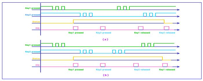
Fig. 3. (a) Two keys pressed, case 1 (b) Two keys pressed, case 2
