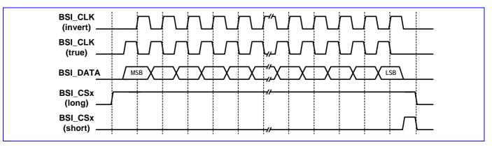
Figure 44 Timing characteristic of BSI interface.
