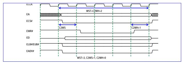
Figure 18 Write Wait State Timing Diagram (ADVW=1)
