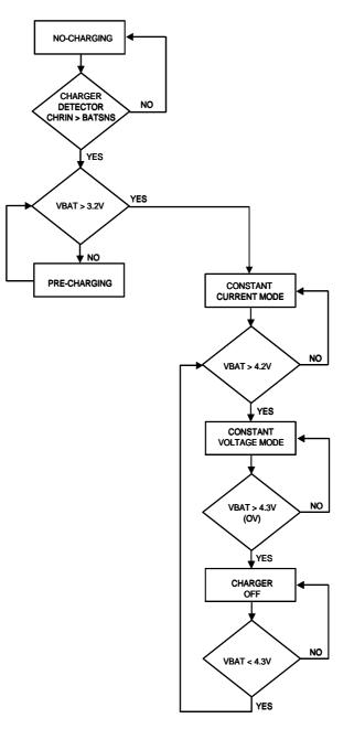
Figure 2. Battery Charger Flow Chart
