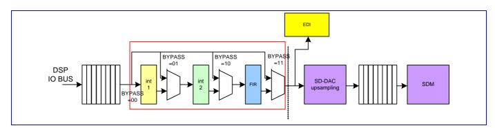
Figure 62 Block diagram of the audio path.
