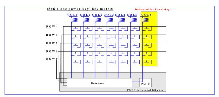
Fig. 1 5x6 matrix with one power-key
