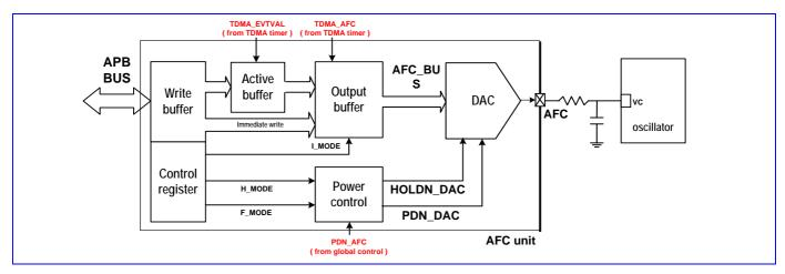
Figure 50 The block diagram of the AFC controller
