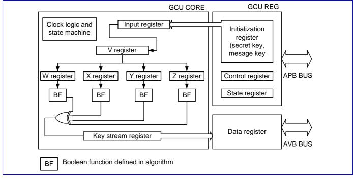
Figure 31 The block diagram of the GCU
