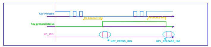
Fig. 2. One key pressed with de-bounce mechanism denoted
