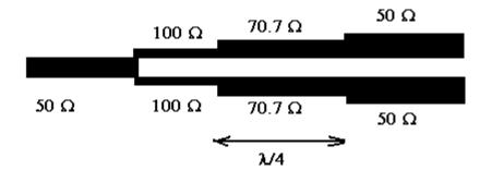
Now, let's consider the length that is required for the 100 ohm lines. They are used to split the power equally and to match to the 50 ohm lines. They can be any length ... any length at all ... including zero length. We can remove them entirely, and just butt the quarter wave transformers up against the input line as shown below, and our system will work exactly the same!
