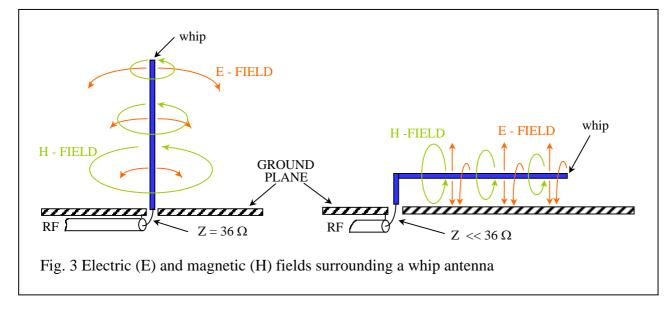
In fig.3 you can see what happens when a quarter wave antenna is bent parallel to ground : apart from the reduction of the radiating impedance (with a mismatch to the transmitter output opt. impedance), what is more important is the modification of the electric field.
