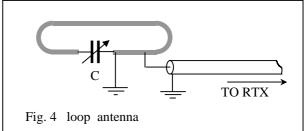
The "loop" antenna must be designed to resonate to the working frequency with a capacitor (fig. 4).
