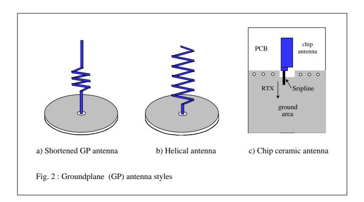
The ground – plane antenna has ( at the resonance frequency ) a nominal impedance of 36  $\Omega$  , which is close enough to the standard 50  $\Omega$  impedance.
