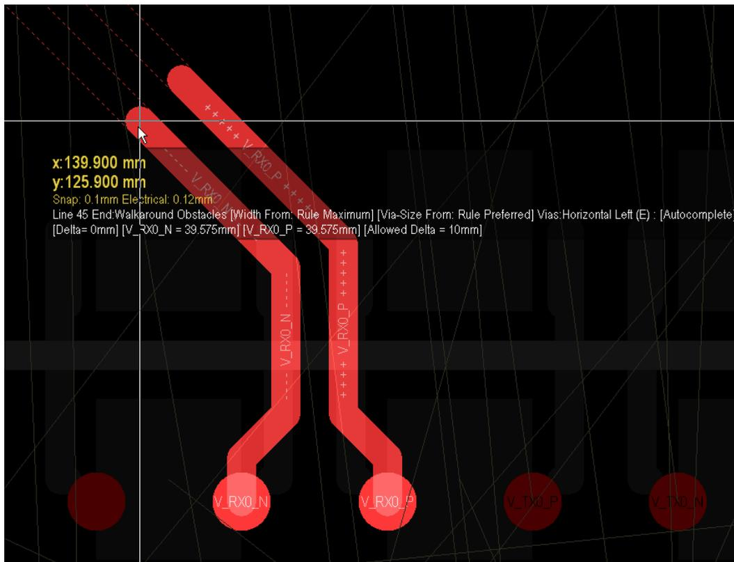
Figure 24. Both nets in the differential pair are routed simultaneously.
