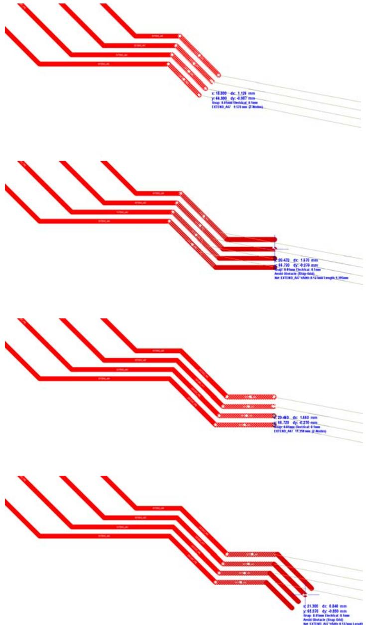
Figure 11. Smart dragging multiple traces – use it to quickly build up a bus of any width, using successive drags of selected track ends.
