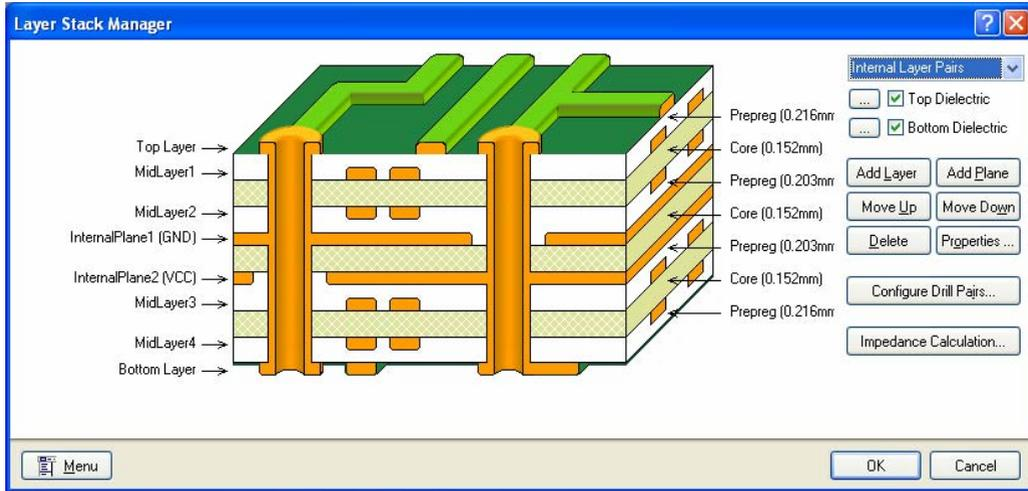
Figure 4. Electrical layers are added in the Layer Stack Manager.
