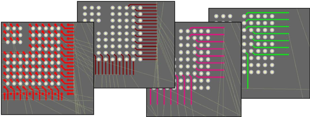
Figure 25. Note how the escape route feature presents each connected pad as an accessible route outside the edge of the BGA.
