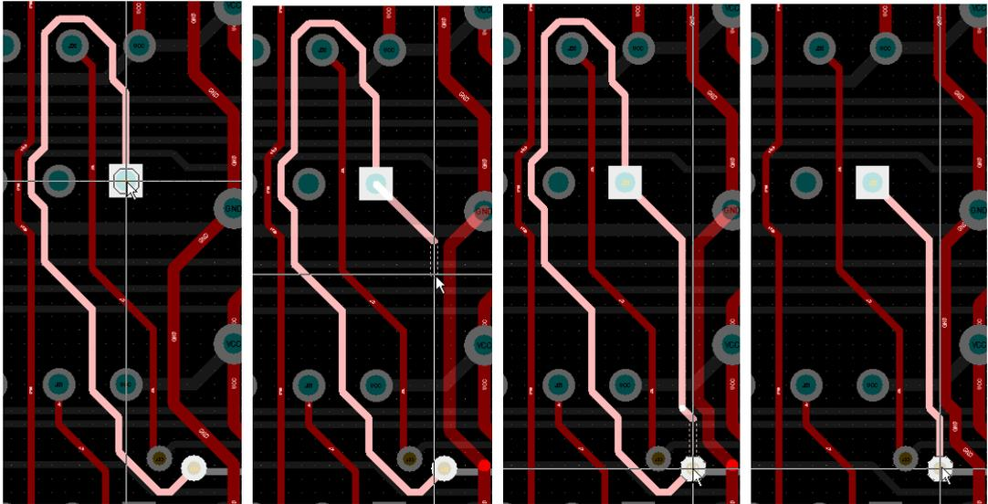
Figure 9. Re-routing an existing route, using push and shove. The old loop is automatically removed.
