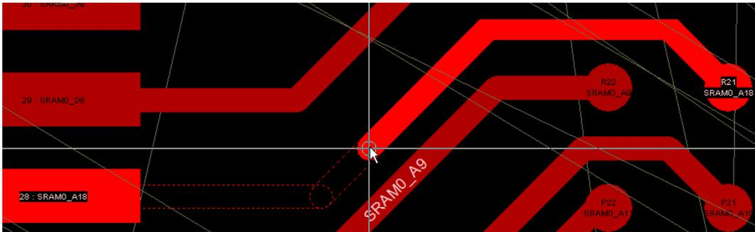
Figure 13. A set of connections being Smart Routed, each requiring just a single click to completely route that connection. Press the tilde key to display the Smart Interactive Routing shortcuts menu during routing.
