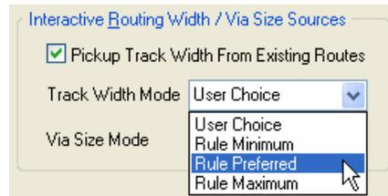
Figure 14. Specify which width should be used when you start routing a net.
