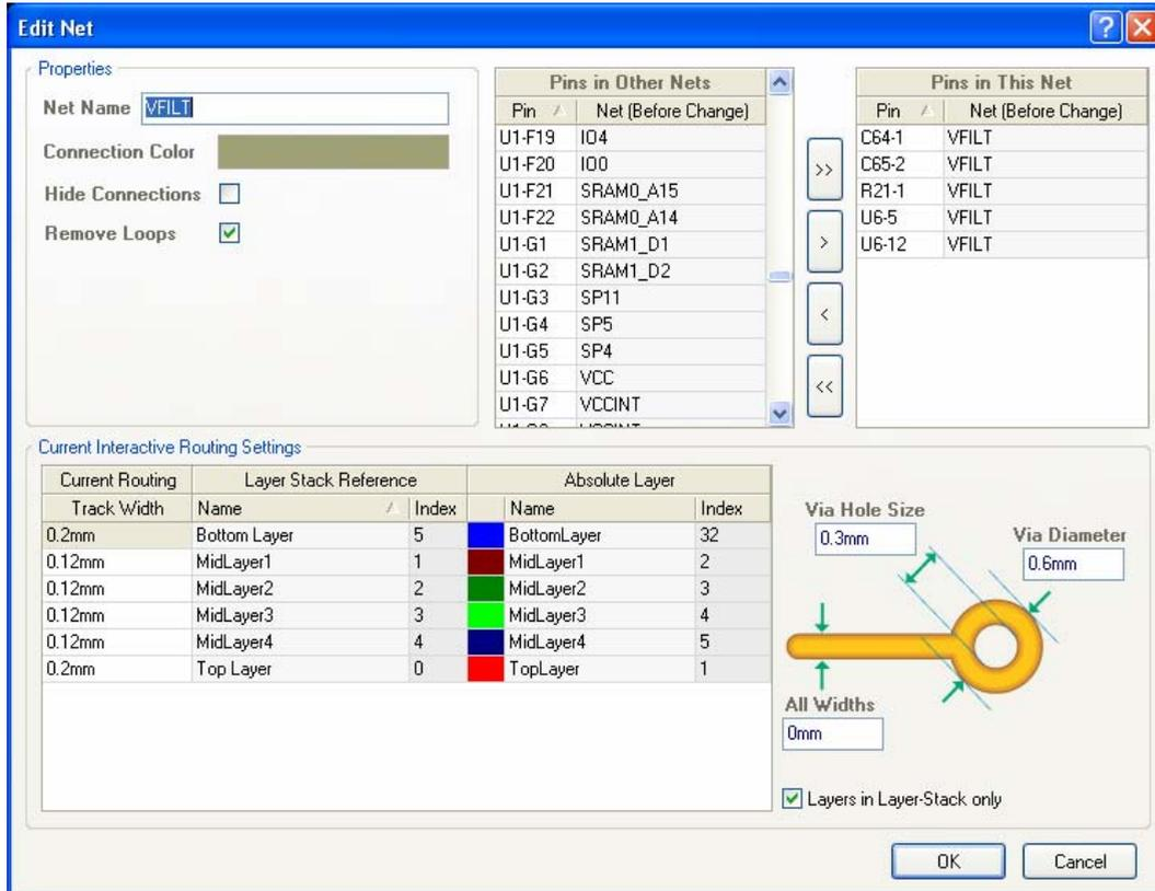
Figure 17. The *Edit Net* dialog can store user-preferred interactive routing track width settings, for this net.
