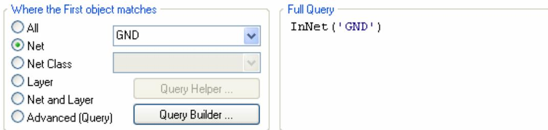
Figure 3. The scope of the rule is specified by entering a query that defines what objects this rule will target..
