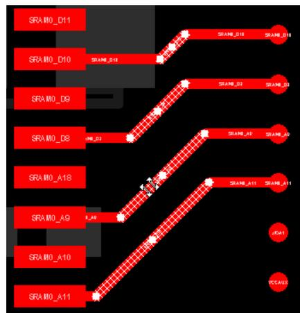
Figure 10. Selected segments have been dragged to a new location.
