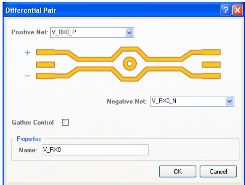
Figure 21. Create a Pair on the PCB using the Differential Pair dialog.
