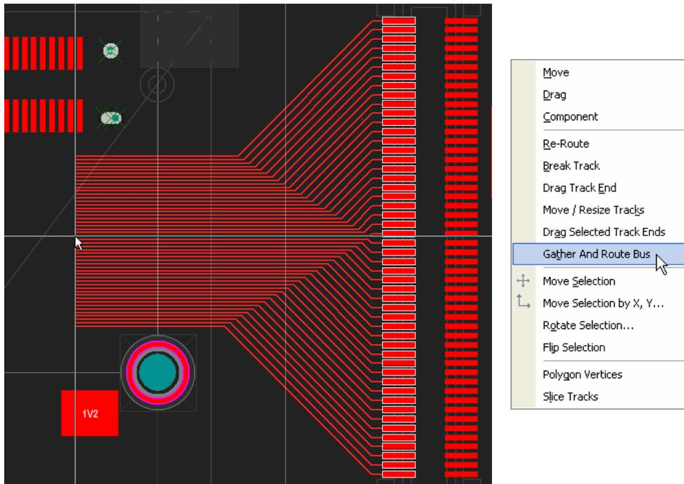
Figure 12. Use the Gather and Route Bus command to start from an unrouted component.
