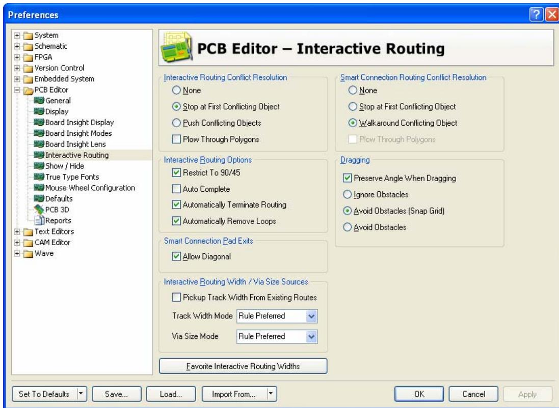
Figure 8. Configure the interactive routing options in the Preferences dialog, or use the Shift+R shortcut and monitor the current mode on the Status bar.
