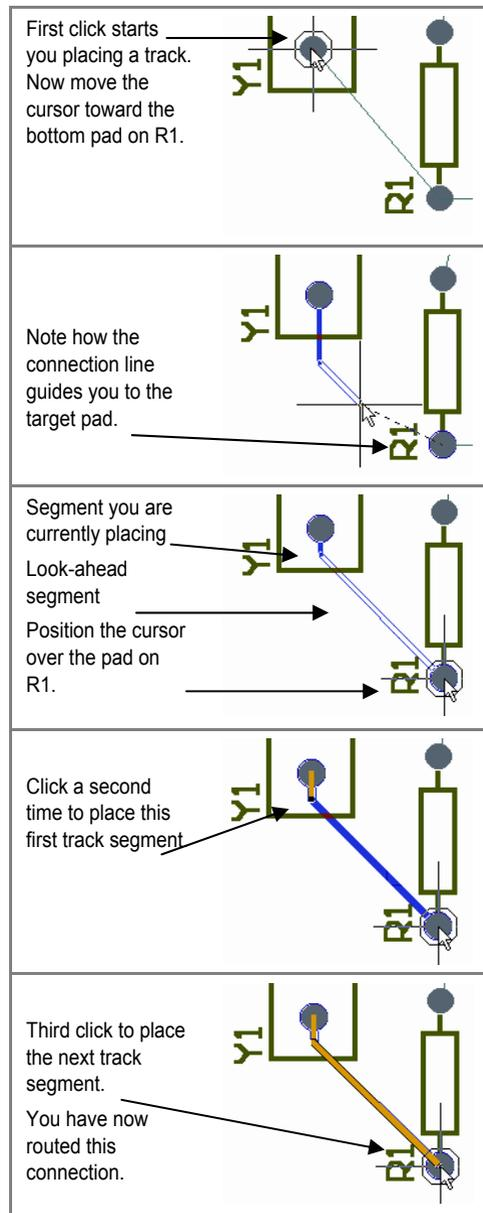
Figure 6. the look-ahead feature allows you to predict the correct location of the current segment, using the next segment.
