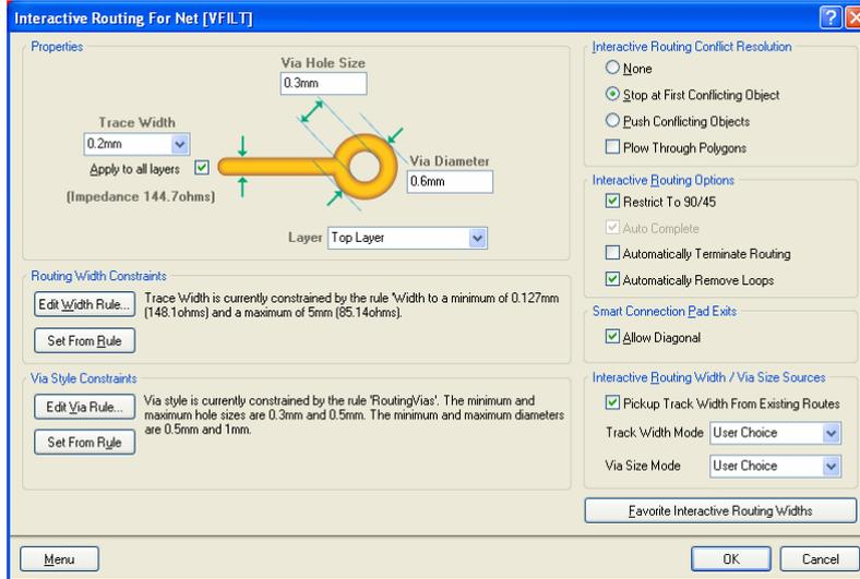
Figure 18. Press **Tab** while routing to open the *Interactive Routing* dialog, where you can enter the routing width.
