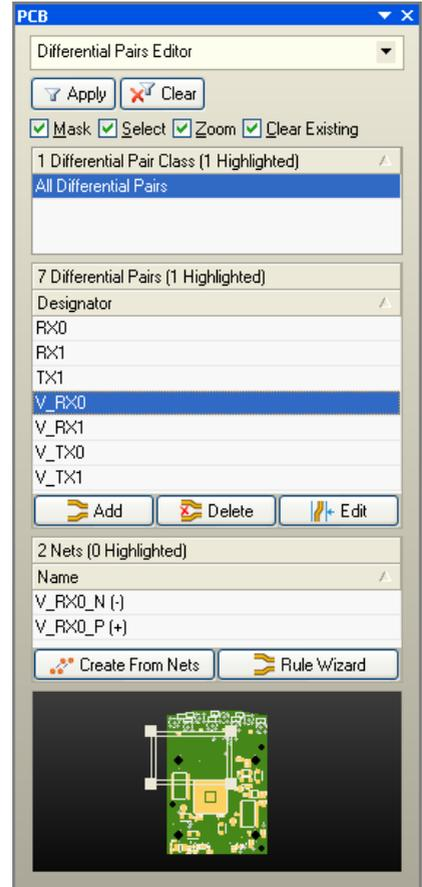
Figure 23. Differential pairs can be viewed and managed in the Differential Pair Editor.
