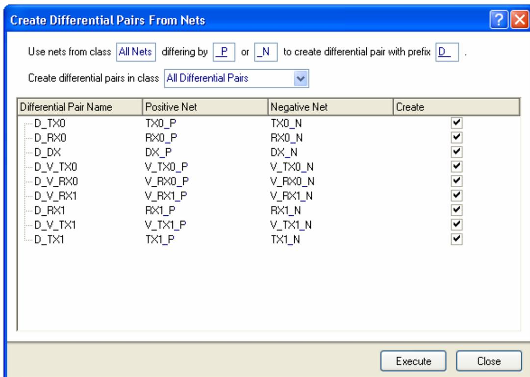
Figure 22. Quickly create pairs for the entire board, based on logical net naming.
