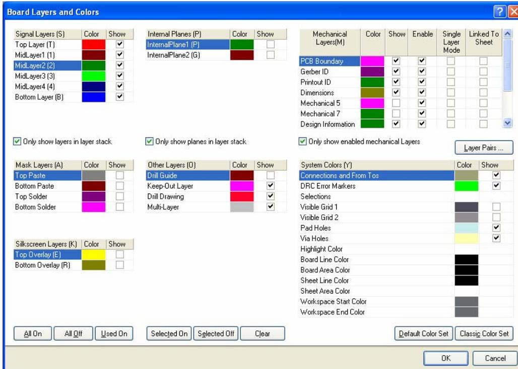
Figure 5. The display of all layers is controlled in the Board Layers and Colors dialog.
