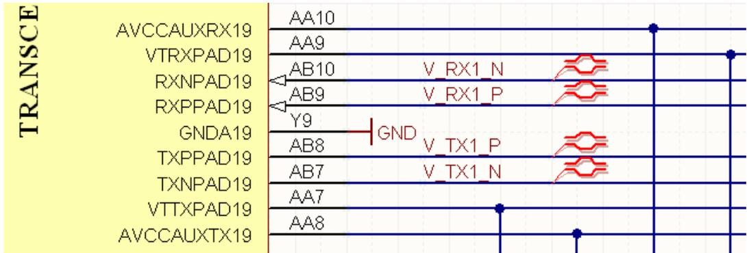
Figure 20. Place Directives on the schematic to define differential pairs.
