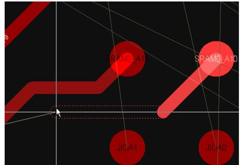
Pushing obstacles, existing routing is moved.
