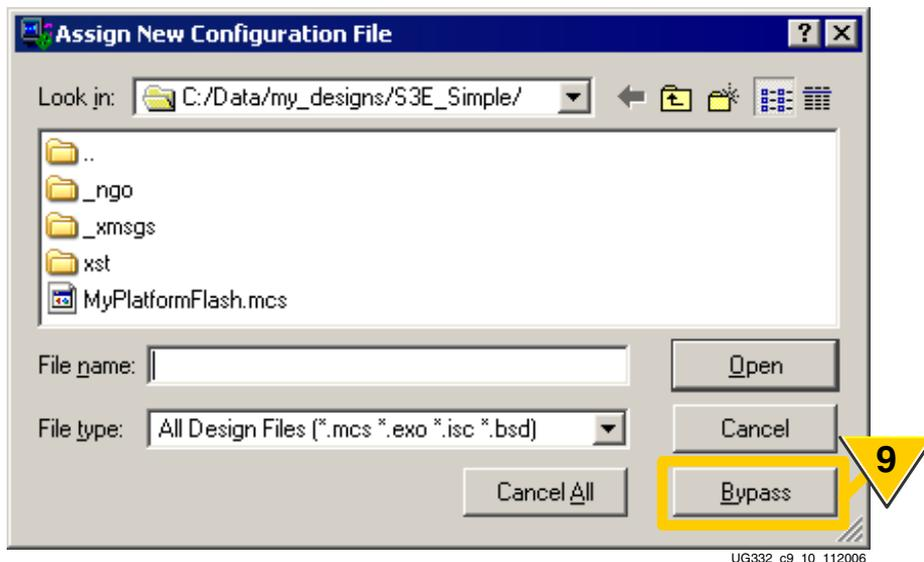
Figure 9-12: Click Bypass to Skip Platform Flash Programming
