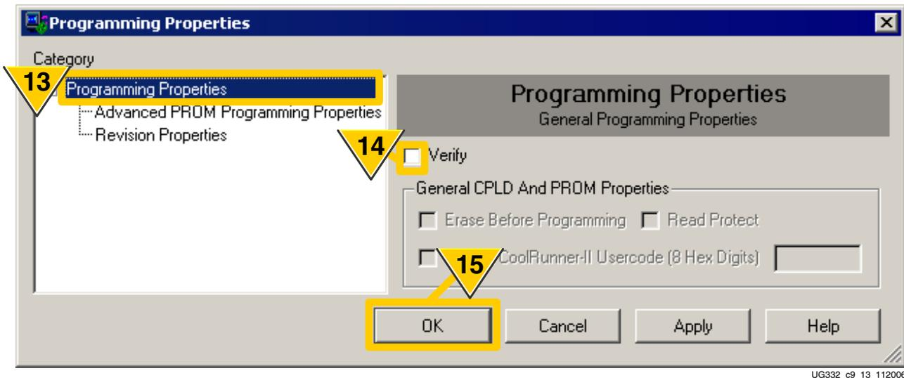
Figure 9-15: FPGA Programming Options
