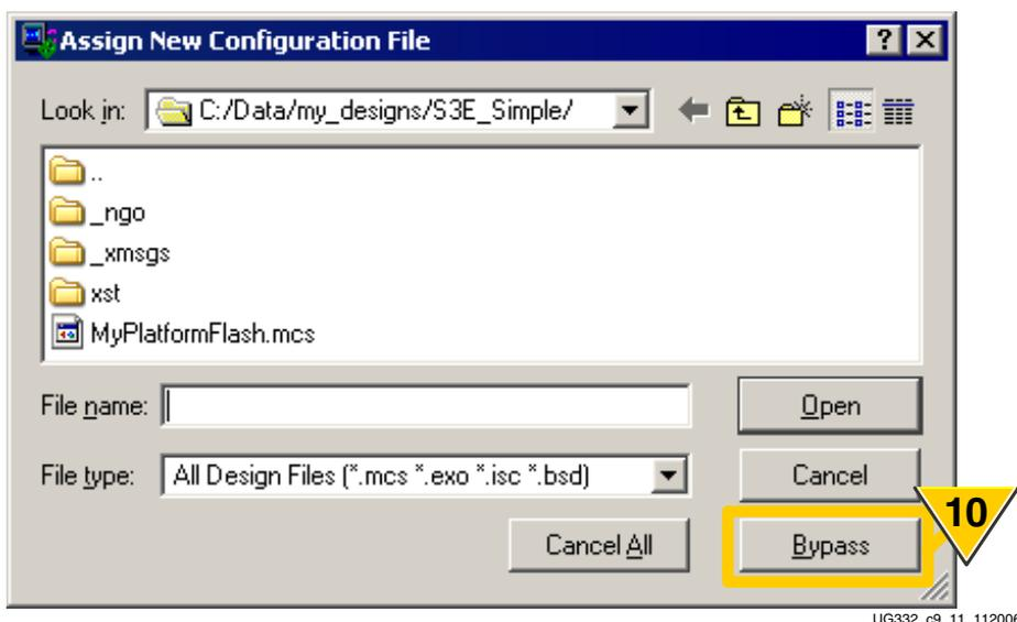
Figure 9-13: Click Bypass to Skip CPLD Programming
