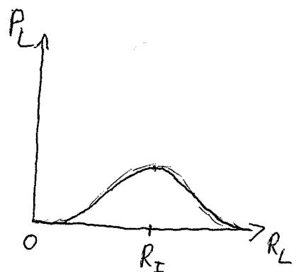
$$\frac{d P_L}{d R_L} = 0 \quad \text{wenn Zähler} = 0 \quad \Rightarrow \quad (R_I + R_L) - 2R_L = 0$$
