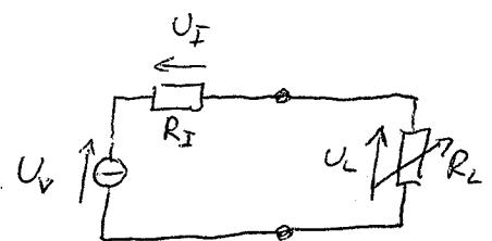
$$\frac{d P_L}{d R_L} = U_V^2 \cdot \frac{1 \cdot (R_I + R_L)^2 - R_L \cdot (2R_L + 2R_I)}{(R_I + R_L)^4}$$
