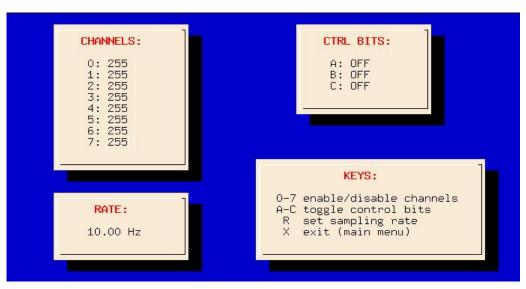
In this mode the user can watch the values of input voltages on selected channels. Channel selection toggled with keys [0] through [7], control bits (relays in fan-out box) are controlled with [A] - [C] keys, acquisition rate is set with the [R] key.
