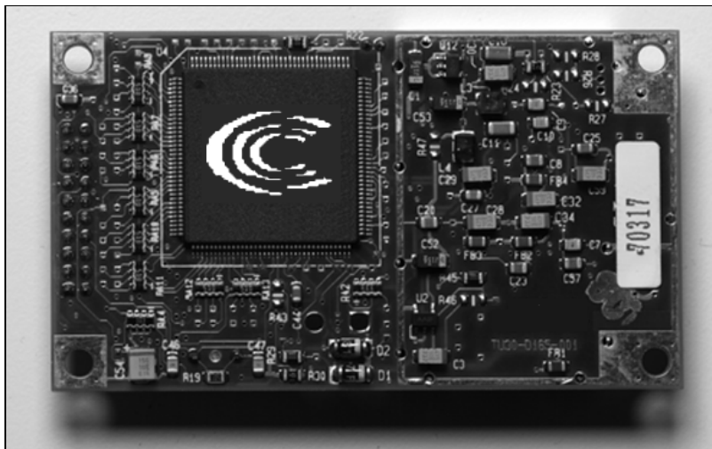
Figure 2. The Conexant Jupiter LP GPS Receiver With Straight OSX RF Connector (Bottom View -- Shown Approximately 1.5x Actual Size)
