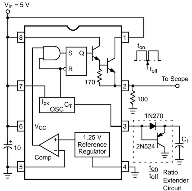
Figure 19. Output Switch On-Off Time Test Circuit
