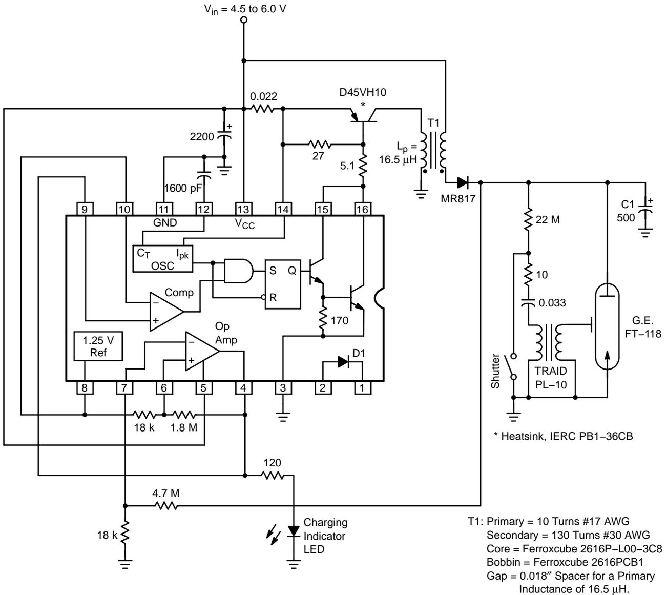
With  $V_{in}$  of 6.0 V, this step-up converter will charge capacitor C1 from 0 to 334 V in 4.7 seconds. The switching operation will cease until C1 bleeds down to 323 V. The charging time between flashes is 4.0 seconds. The output current at 334 V is 45 mA.
