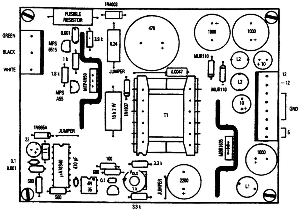
Printed Circuit Board Negative – Bottom View
