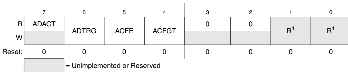
Figure 10-5. Status and Control Register 2 (ADCSC2)
