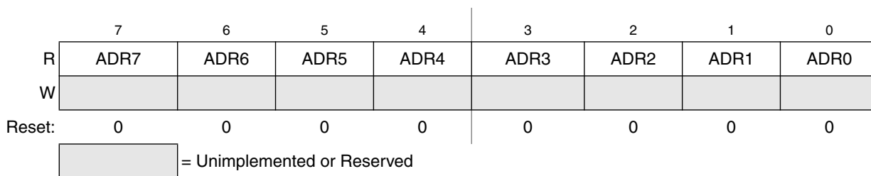
Figure 10-7. Data Result Low Register (ADCRL)
