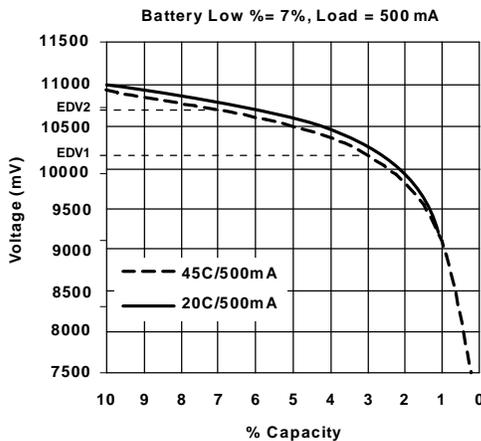
Figure 11. EDV Calculations vs Capacity for Various Temperatures
