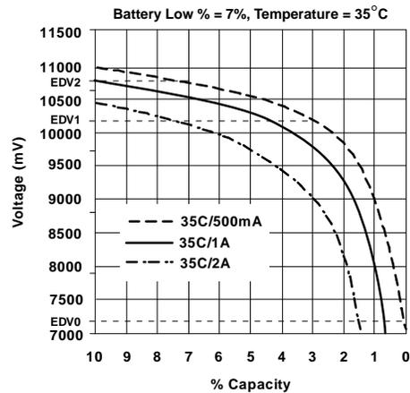
Figure 12. EDV Calculations vs Capacity for Various Loads
