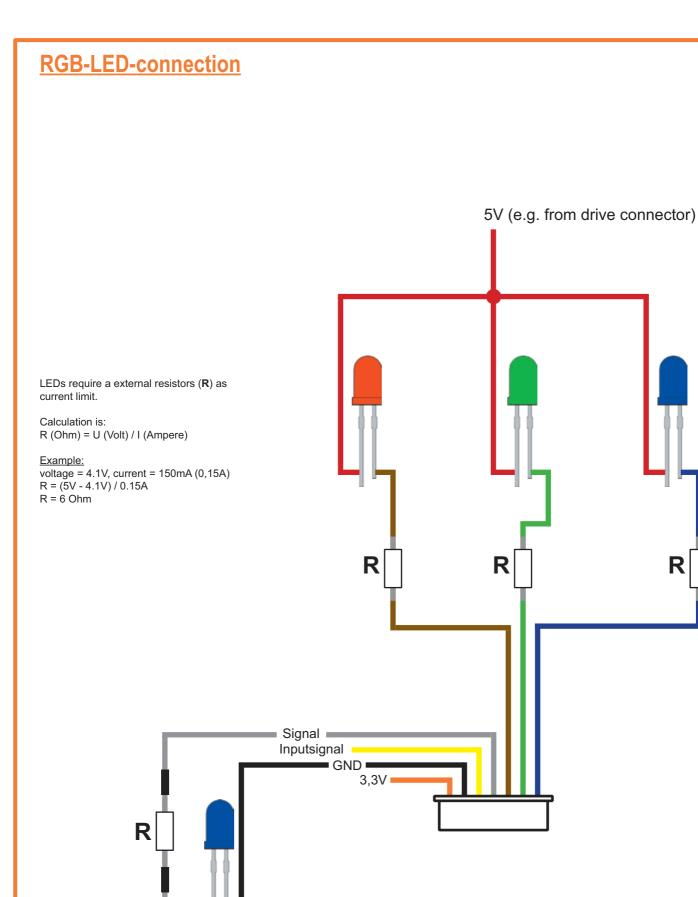
An additional extern status-LED, which shows the current state of the SmartXX, can be connected.
