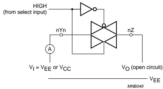
Fig.10 Test circuit for measuring ON-state current.
