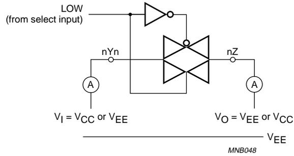
Fig.9 Test circuit for measuring OFF-state current.
