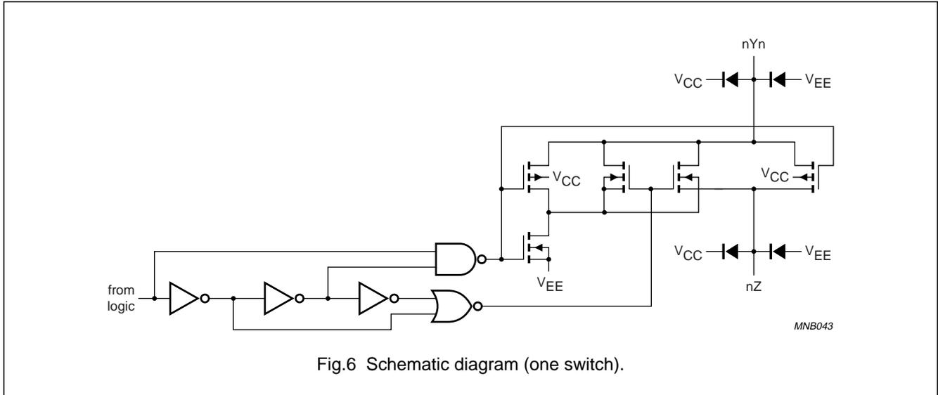
Fig.6 Schematic diagram (one switch).
