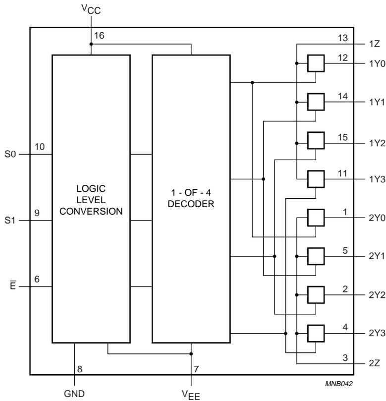
Fig.5 Functional diagram.
