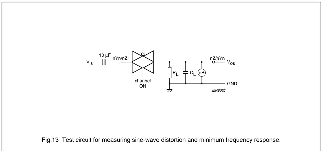
Fig.13 Test circuit for measuring sine-wave distortion and minimum frequency response.
