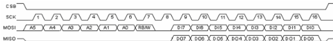
Figure 9. SPI frame format for two 8 bit words.
