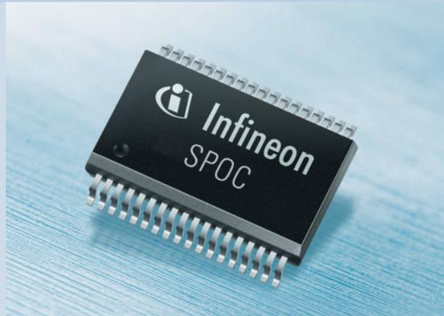
THE SPOC products are five channel high-side smart power switches in P-DSO-36-20 package providing embedded protective functions. They are especially designed to control standard exterior front and rear lighting in automotive applications.
