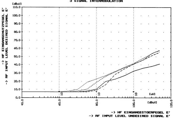
3-SENDER-INTERMODULATION 3 SIGNAL INTERMODULATION
