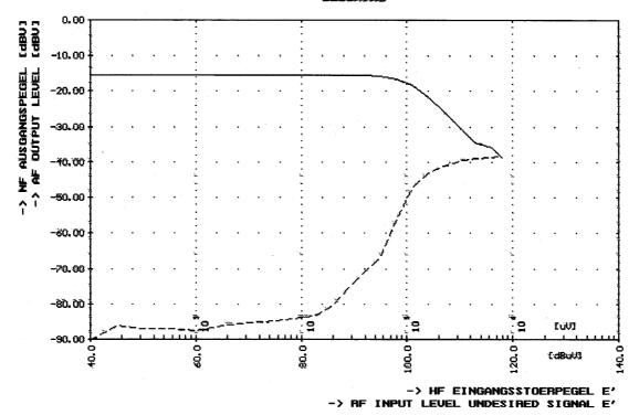
Us = 8.5 V fmod= 1.0 kHz Dev = ±22.5 kHz f = 95.550 MHz undesired f = 95.200 MHz desired E' = 20 µV desired Audio Bandpass ikHz ±22.5 kHz Noise
