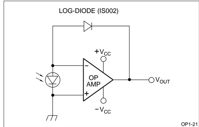
**Figure 5. Logarithmic Photocurrent Amplifier using an Operational Amplifier**
