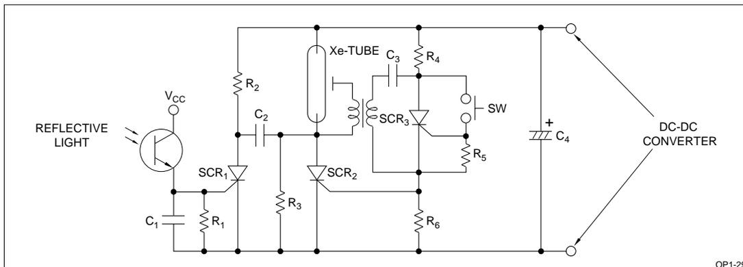
Figure 14. Auto-Stroboscope Circuit
