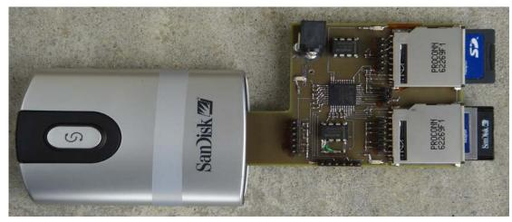
Figure 7: Demo Board Plugged into USB SD Card Reader
