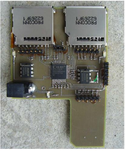
Figure 6: SD Multiplexer Demo Board
