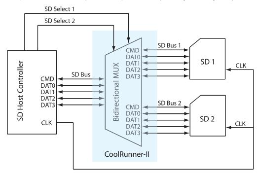
Figure 3: Block Level Diagram: A Bidirectional Multiplexer
