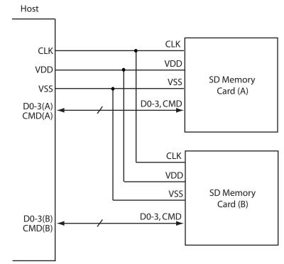
Figure 2: SD System Bus Topology
