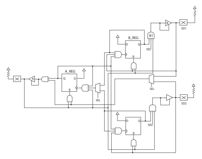
Figure 4: SD Multiplexer Circuit for Two SD Devices
