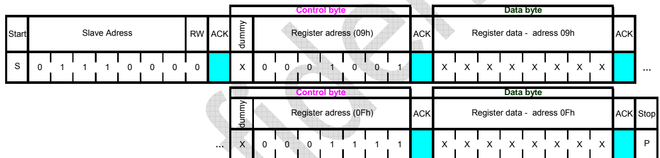
Figure 15: I 2 C multiple write protocol
