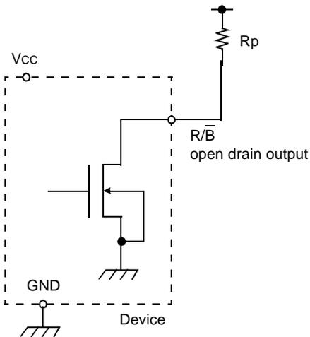
$$R_p = \frac{V_{cc}(\text{Max.}) - V_{OL}(\text{Max.})}{I_{OL} + \sum I_L} = \frac{3.2V}{8\text{mA} + \sum I_L}$$
