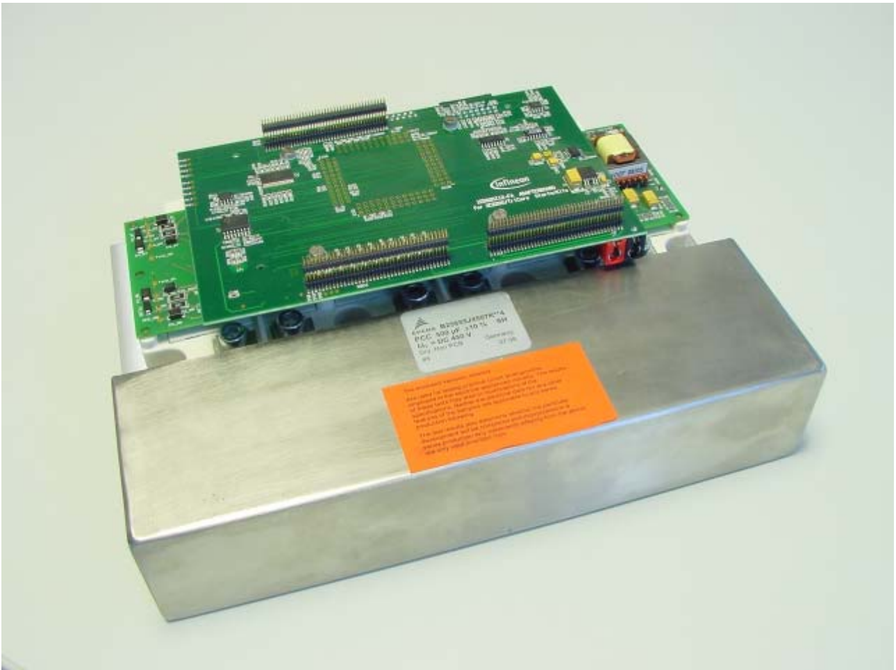
Figure 61 Adapter board connected to the 6ED100HP2-FA driver board and fixed by means of spacers and screws
