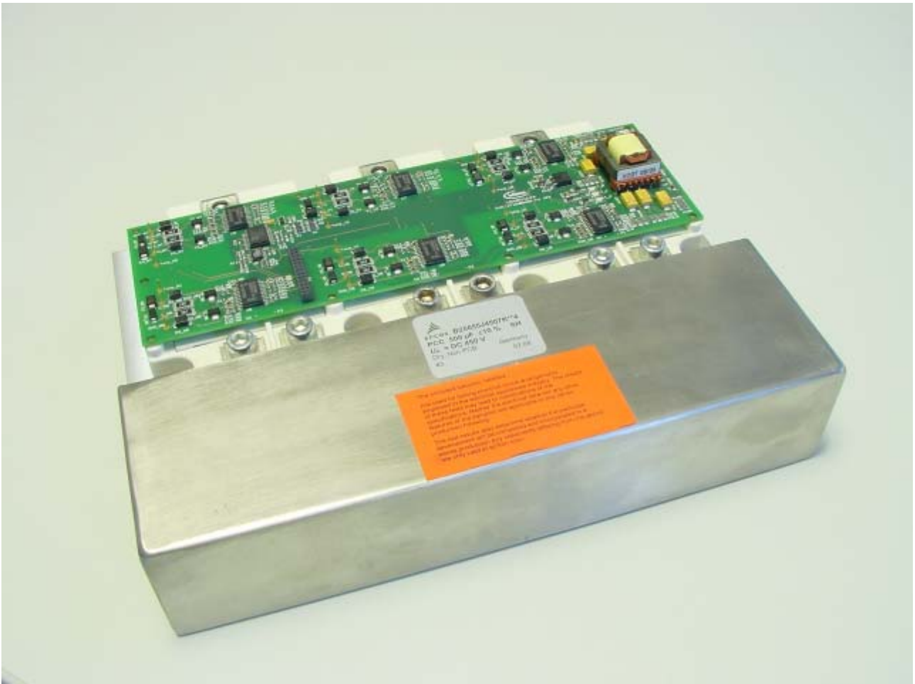
Figure 60 DC-Link capacitor screwed to HybridPack2™ terminals
