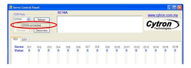
n. Now, Servo Control Panel is ready to control the servo motor on SC16A, please ensure the power for servo motor is connected properly.
