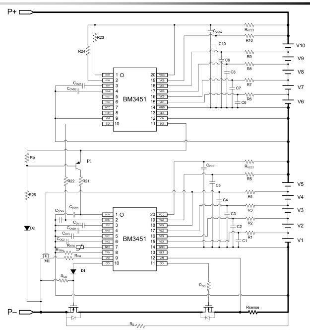
Figure 8 10-cell application—without balance function
