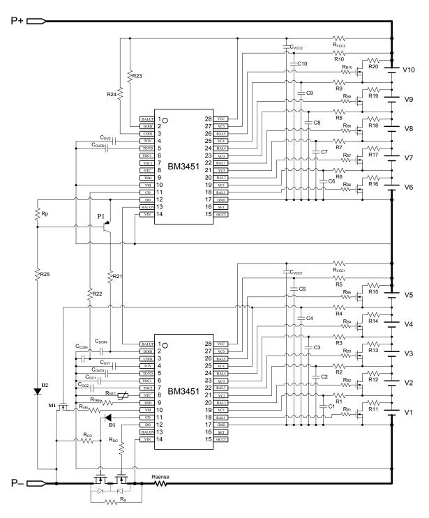
Figure 7 10-cell application—with balance function
