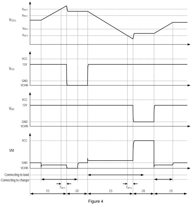
Assuming the charging current is constant, VCHR- is the voltage of the charger's negative terminal:
