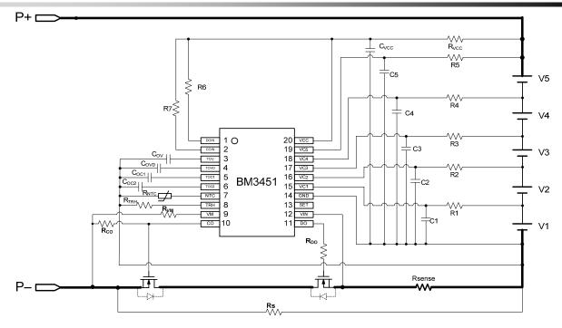
Figure 6 (d-1) 5-cell application (SET floating)
