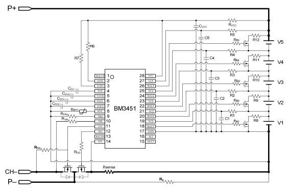
Figure 6 (a-2) **5-cell application (SET floating)**---with balance function, charge and discharge circuits separated
