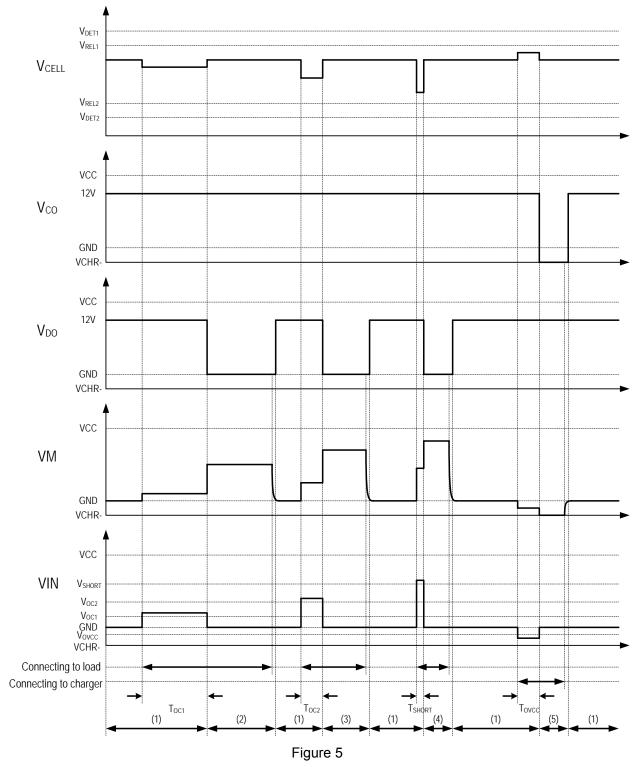
Assuming the charging current is constant, VCHR- is the voltage of the charger's negative terminal:
