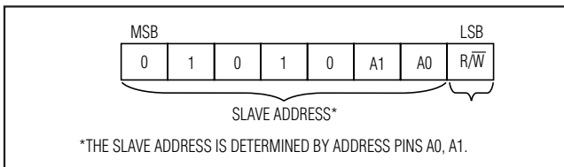
Figure 1. DS3502 Slave Address Byte
