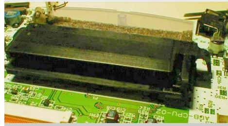
To the right, we see the extension slot. It is the same as the one in all previous GameBoy's. Power, Ground, 8 data and 16 address lines. Plus some control lines. That's it. The GBA will gladly accept GameBoy cartridges and run with them as well. The GBA senses the
