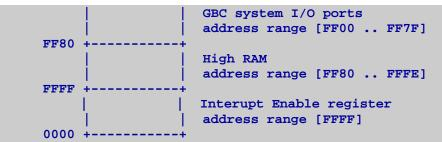
The **address range** consists of the addresses that are possible in that section of memory. The first number is the first possible address and the second number (the one after the two dots) is the LAST address of that range. It is INCLUSIVE. People aquainted with Modula-2 will be familiar with this notation.
