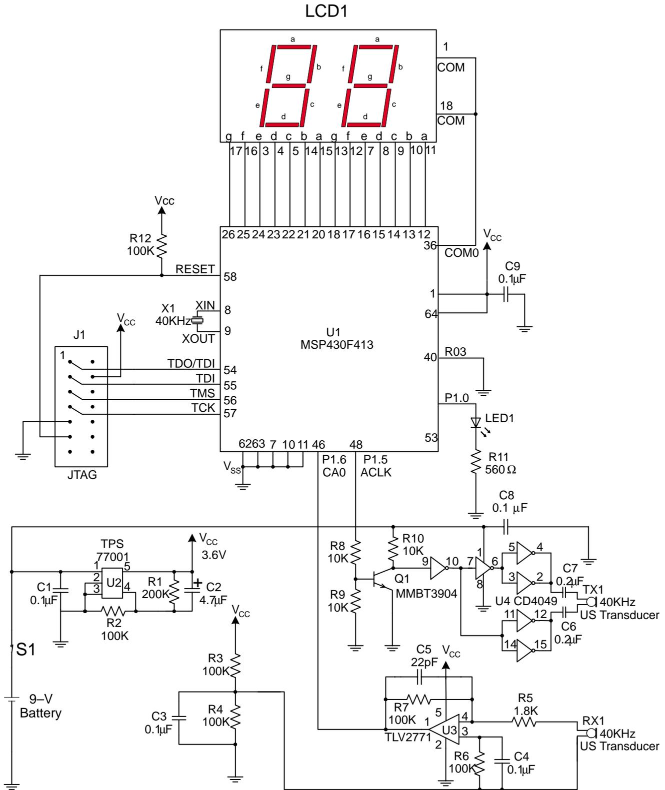
**Figure 1. Circuit Schematic**
