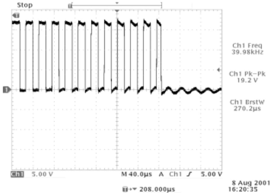
Figure 2. Oscilloscope Trace of Transmitter's 40-kHz Burst
