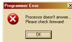
Illustration 3: Firmware is missing in the programmer
