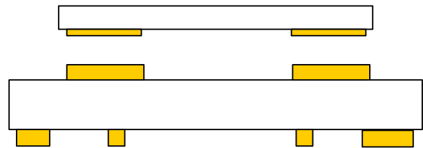
Figure 20. Correct PCB Top Metal Pattern Under Package
