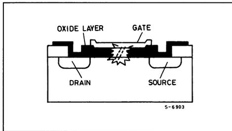
This happens mostly because a charged conductor, typically a person, is rapidly discharged through the device.
