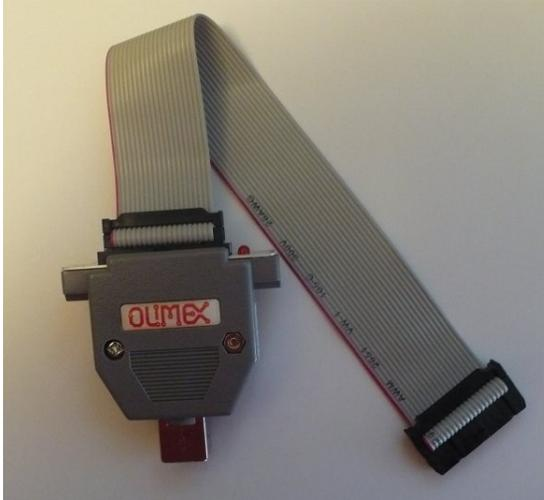
The device used with this tutorial is the [ARM-USB-TINY](#) which costs \$41.00. You could use something different like the [ARM-USB-JTAG](#) which costs \$72.00. Unless you need the extra serial port and need the power supply this device has no real advantage over the tiny device.
