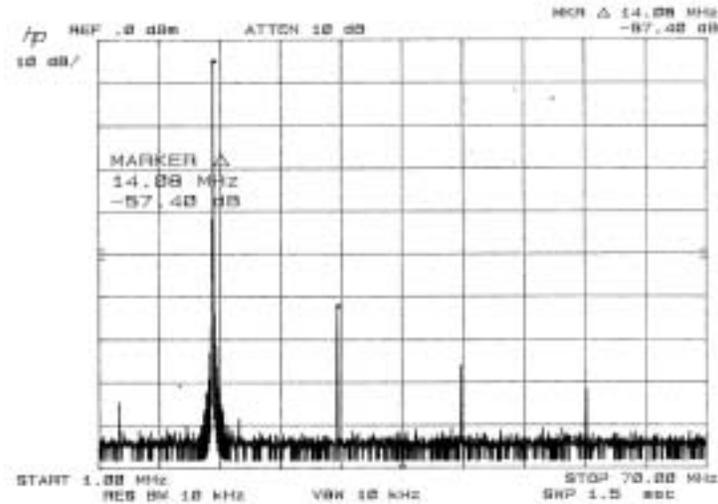
**FIGURE 19: DEIC420 14 MHZ SPECTRUM (WITH FILTER)**
