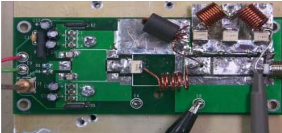
**FIGURE 18: DEIC420 14 MHZ MODULE (WITH FILTER)**
