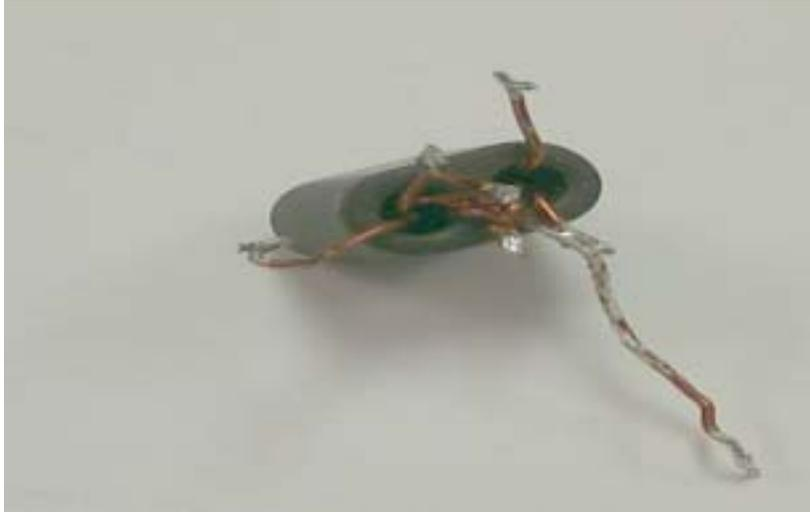
**FIGURE 20: T1, 25:1, MULTI-FILAR AUTOTRANSFORMER**
