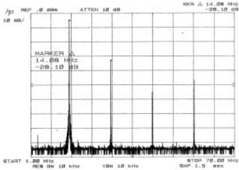
**FIGURE 12: DEIC420 14.0 MHZ SPECTRUM (NO FILTER)**
