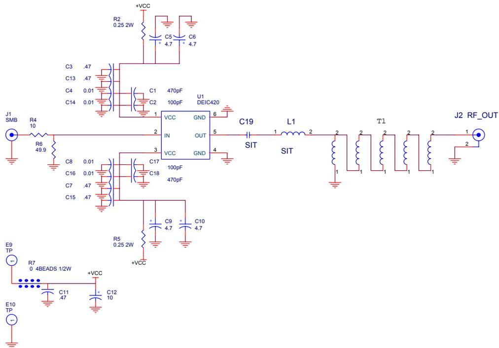
**FIGURE 2: DEIC420 RF DRIVER SCHEMATIC DIAGRAM**
